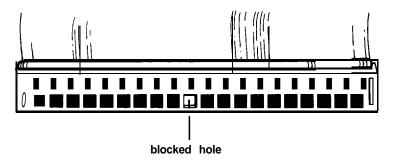
7. Pick up the hard disk drive that you removed from the vertical mounting position. Notice the ribbon cable socket on the back of the drive; you see two rows of pins. In one of the rows, a pin is missing.
